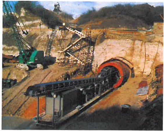
The Mersey Mole is a tunnelling machine designed for excavating soft rock. It was used in 1967 to cut a 10.3m diameter
