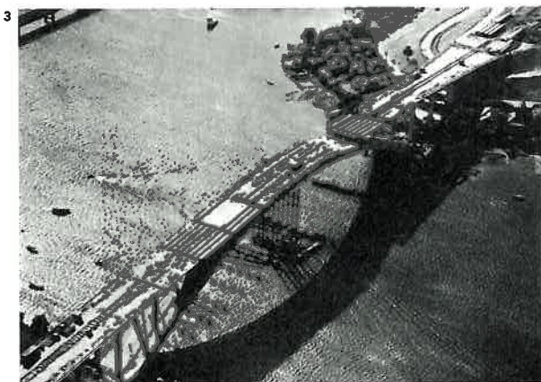
3 The Gladesville Bridge over the Parramatta River at Sydney, Australia, is a 305m span concrete arch with a height of 41m. It was formed from pre-cast elements erected on a steel centring.
